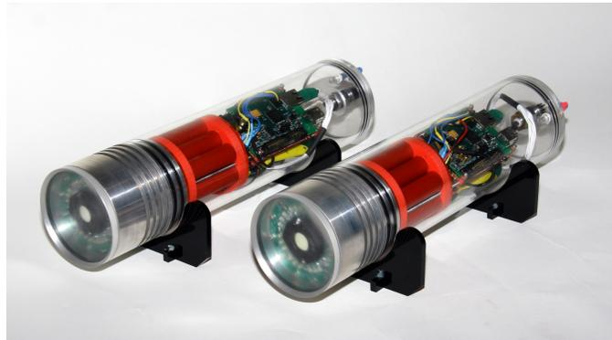
Fig. 1. Two AquaOptical II modems.
