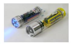
A previous version of the Aqua-OpticalLong receiver used a variable gain amplifier (VGA) in conjunction with an analog threshold filter to digitize the incoming signal. We replaced this setup with the ADC and the first stage FPGA. In the experimental section of this article, we refer to this previous version as the AquaOpticalLong with VGA. We refer to the new version as AquaOpticalLong with MF.
