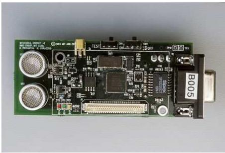
Fig. 2. The Cricket sensor node.
