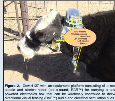
Figure 2. Cow 4127 with an equipment platform consisting of a neck saddle and stretch halter (ear-a-round, EAR™) for carrying a solar powered electronics box that can be wirelessly controlled to deliver directional virtual fencing (DVF™) audio and electrical stimulation cues.
